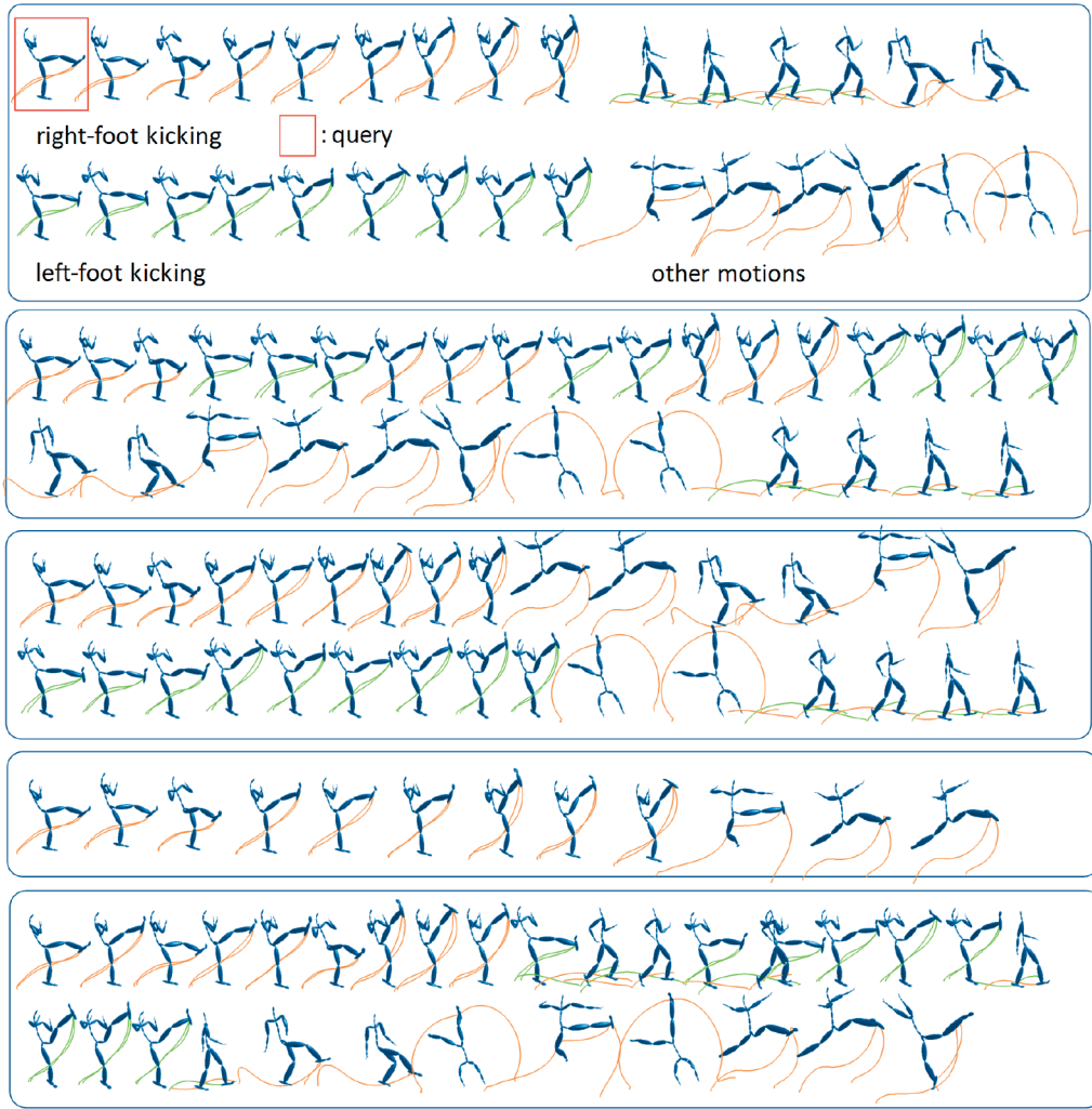
Fig. 14. The evaluation of motion retrieval. First row: the selected data set; second and third rows: our approach using the coefficients of the lower part in level 2 and the lower limbs in level 3, respectively. The weights for other parts are set to 0.0; fourth row: retrieve by using geometric relations [13]. The geometric relations F_l^3 , F_l^4 (left/right foot raised, refer to [13, Table 1]) and F_l^7 , F_l^8 (left/right knee bent) are selected; fifth row: retrieve by using DTW. The clip marked by red rectangle is the query. The trajectories of right foot and left foot are displayed by red and green colors, respectively.
